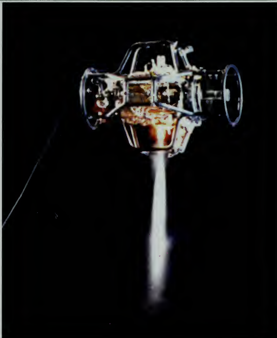
Fig. 3-30. State of the art technology is proven as the Lightweight Exoatmospheric Projectile tracks a simulated target in this hover test.
